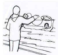
For a 22"/24" lifebuoy the holder normally contains 20m of buoyant line
